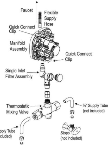
Control Module with Single Inlet Tee Filter Assembly and Below Deck Thermostatic Mixing Valve (BDT)
