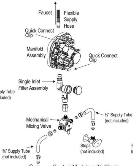
Control Module with Single Inlet Tee Filter Assembly and Below Deck Mechanical Mixing Valve (BDM)
