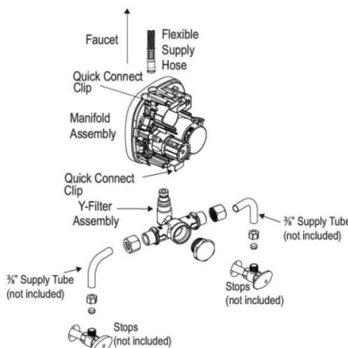
Control Module with Double Inlet Tee Filter Assembly.
